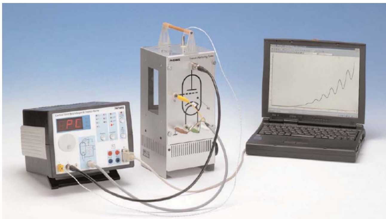
Fig.1: Set-up for the Franck-Hertz experiment with PC.
