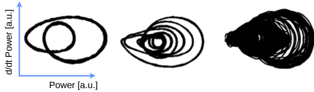
FIG. 40 (color online). The transition toward chaotic motion in an optomechanical system has been observed by Carmon, Cross, and Vahala (2007) (courtesy of Tal Carmon).
